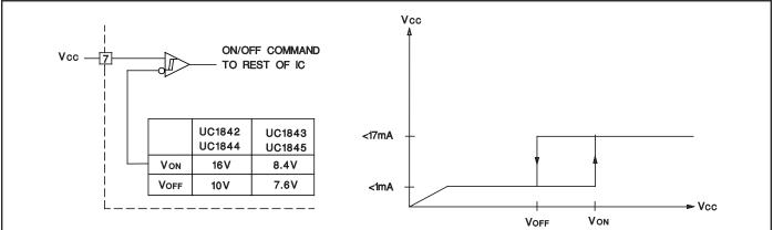
During under-voltage lock-out, the output driver is biased to sink minor amounts of current. Pin 6 should be shunted to ground with a bleeder resistor to prevent
