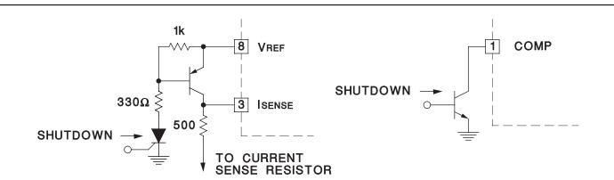
Shutdown of the UC1842 can be accomplished by two methods; either raise pin 3 above 1V or pull pin 1 below a voltage two diode drops above ground. Either method causes the output of the PWM comparator to be high (refer to block diagram). The PWM latch is reset dominant so that the output will remain low until the next
