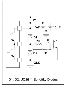
**Power Bipolar Drive Circuit**
