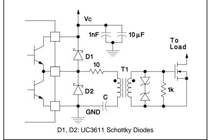
**Transformer Coupled MOSFET Drive Circuit**
