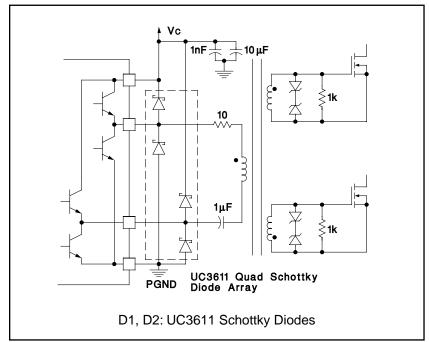
**Transformer Coupled Push-Pull MOSFET Drive Circuit**
