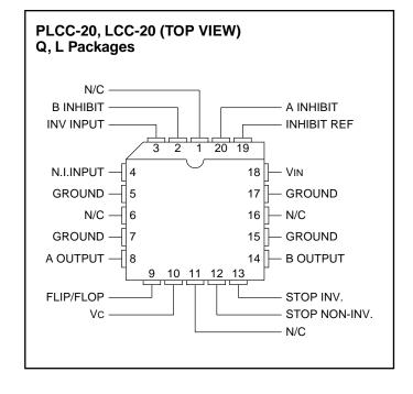
Note: All four ground pins must be connected to a common ground.
