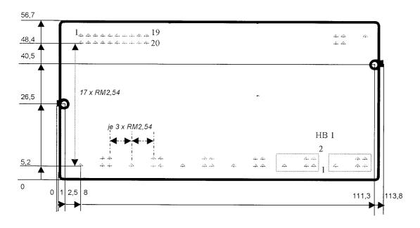
Fig. 9 Dimensional drawing, layout
