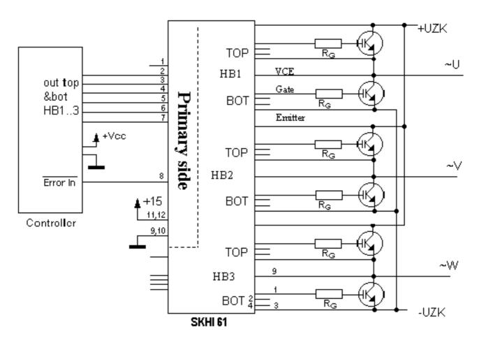
Fig. 7 SKHI 61 block diagram
