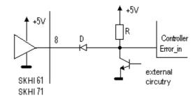
Fig. 2 \_ERR-Signal in an "open-collector"-circuit
