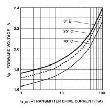
Figure 7. Typical Forward Voltage vs. Drive Current.
