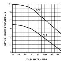
Figure 4. Typical Optical Power Budget vs. Data Rate.
