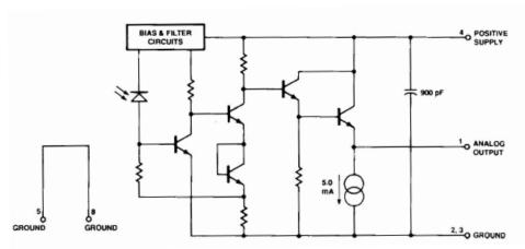
Figure 10. Simplified Receiver Schematic.
