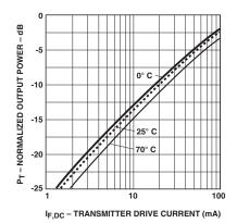
Figure 8. Typical Normalized Output Optical Power vs. Drive Current.
