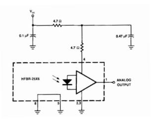
Figure 9. Recommended Power Supply Filter Circuit.
