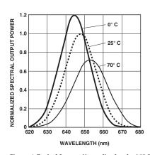
Figure 6. Typical Spectra Normalizedto the 25° C Peak.
