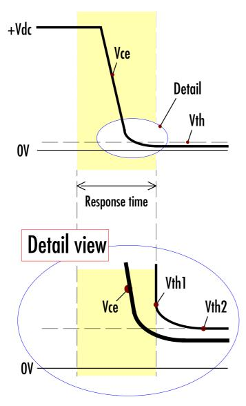
Fig. 5 Collector-sense voltage curve
