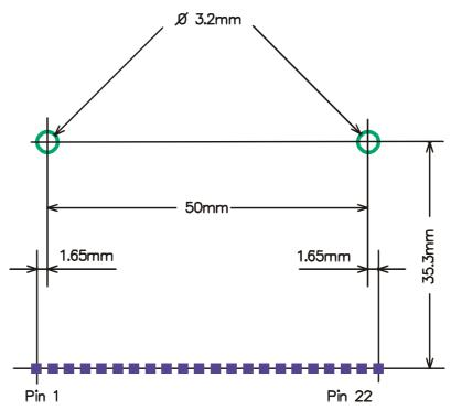
Fig. 3 Side view (top) / Mechanical fixing (bottom) 2SD315AI-33 Height X: typ. 22mm
