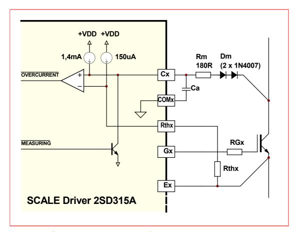
Fig. 4 Collector-sense circuit principle
