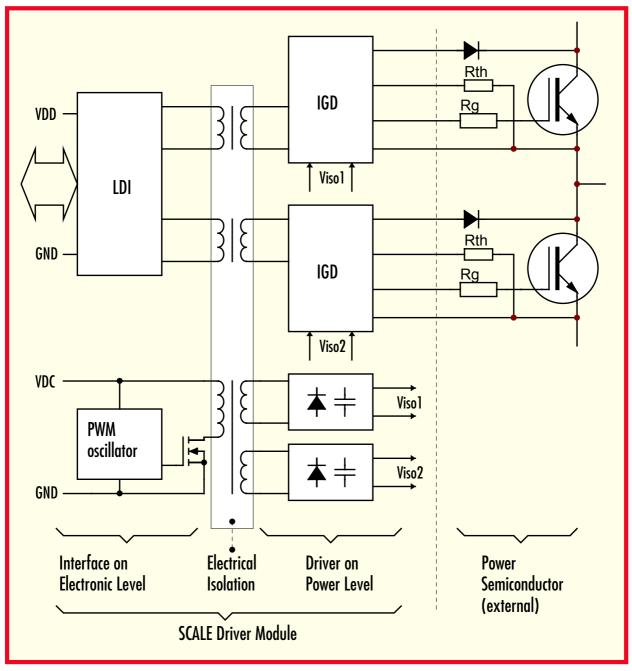
Fig. 1 Block diagram of the 2SD315AI-33
