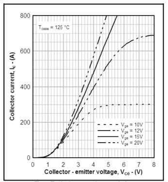
Fig. 4 Typical output characteristics
