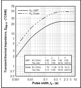
Fig. 10 Transient thermal impedance
