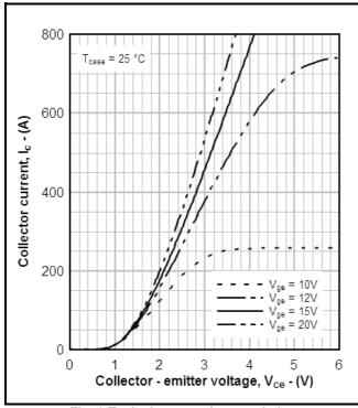
Fig. 3 Typical output characteristics
