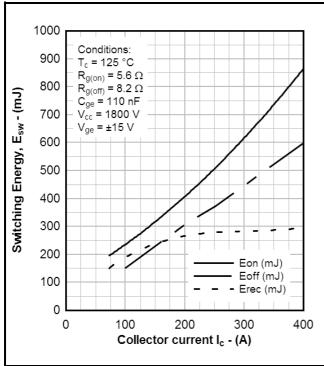
Fig.5 Typical switching energy vs collector current
