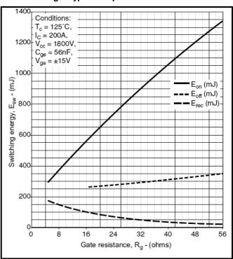
Fig.6 Typical switching energy vs gate resistance
