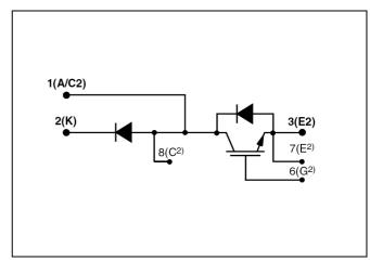
Fig. 1 Chopper circuit diagram
