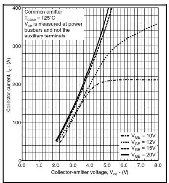
Fig.3 Typical output characteristics
