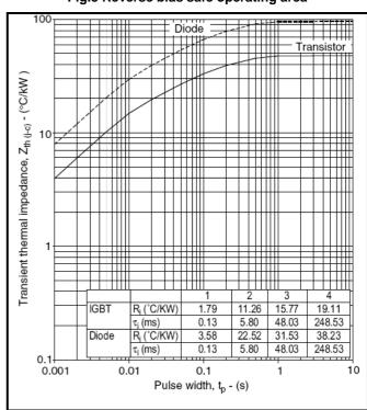
Fig.10 Transient thermal impedance
