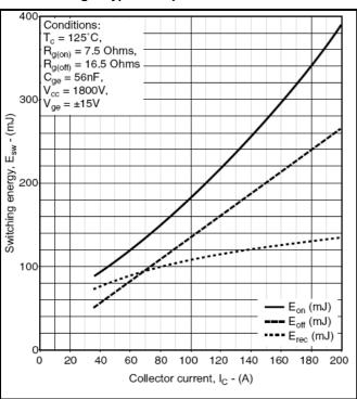
Fig.5 Typical switching energy vs collector current
