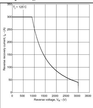
Fig.9 Diode reverse bias safe operating area
