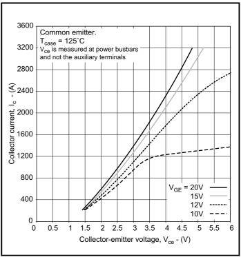
Fig. 3 Typical output characteristics
