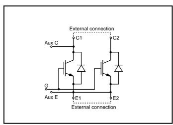
Fig. 1 Single switch circuit diagram
