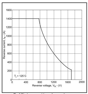
Fig. 9 Diode reverse bias safe operating area
