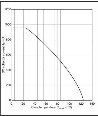
Fig. 10 DC current rating vs case temperature
