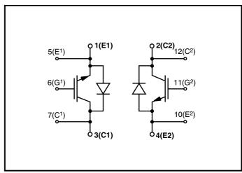
Fig. 1 Dual switch circuit diagram
