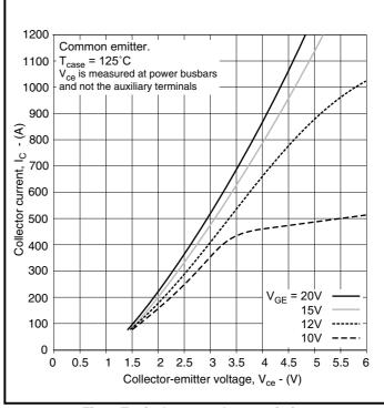
Fig. 3 Typical output characteristics
