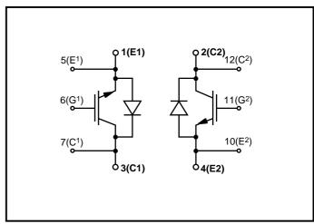
Fig. 1 Dual switch circuit diagram
