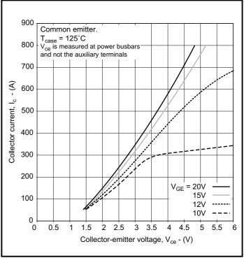
Fig. 3 Typical output characteristics
