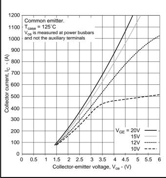
Fig. 3 Typical output characteristics
