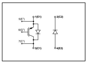
Fig. 1 Chopper circuit diagram
