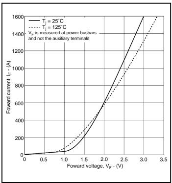
Fig. 6 Diode typical forward characteristics
