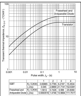
Fig. 10 Transient thermal impedance
