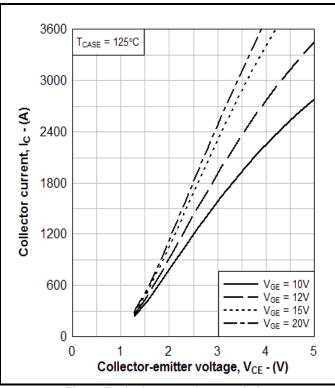
Fig. 4 Typical output characteristics
