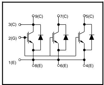
Fig. 1 Circuit configuration
