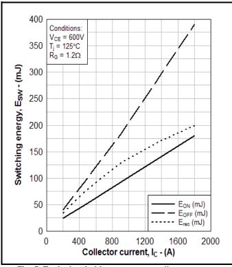
Fig. 5 Typical switching energy vs collector current
