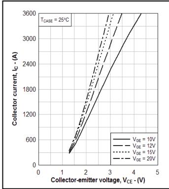
Fig. 3 Typical output characteristics
