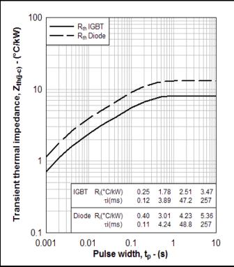
Fig. 10 Transient thermal impedance
