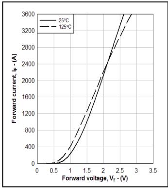
Fig. 7 Diode typical forward characteristics
