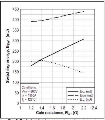
Fig. 6 Typical switching energy vs gate resistance
