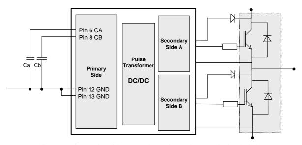
Figure 3.3 Connection of the external capacitors to increase the interlock times
