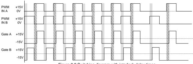
Figure 3.2 Switching diagram with interlock delay times
