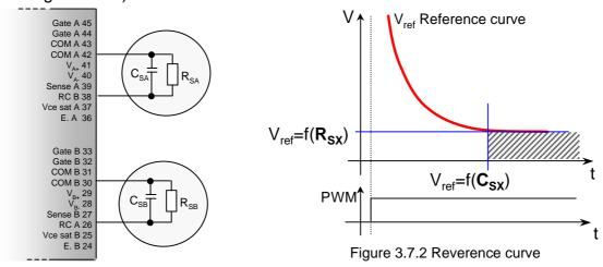
Figure 3.7.1 R<sub>SX</sub> and C<sub>SX</sub> connection to adjust the reference curve
