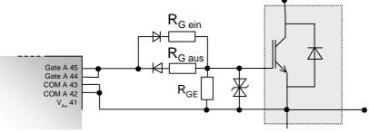
Figure 3.62 Gate connection with  $R_{G \text{ on}}$  and  $R_{G \text{ off}}$
