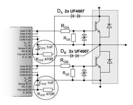
Figure 3.7.4 Trigger suppression of the V<sub>ce sat</sub> measurement
