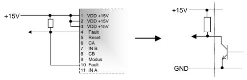
Figure 3.4 Fault output
