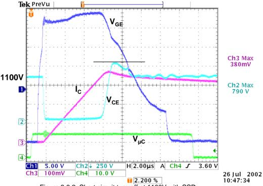
Figure 3.8.2: Short circuit turn-off at 1100V with SSD
