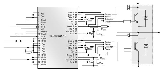
Figure 1.6 Pin configuration of the 2ED300C17-S
