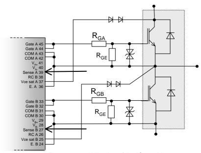
Figure 3.10.1 Utilization of the "Sense" input
