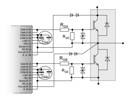
Figure 3.11 2ED300C17-S with external buffer capacitors
