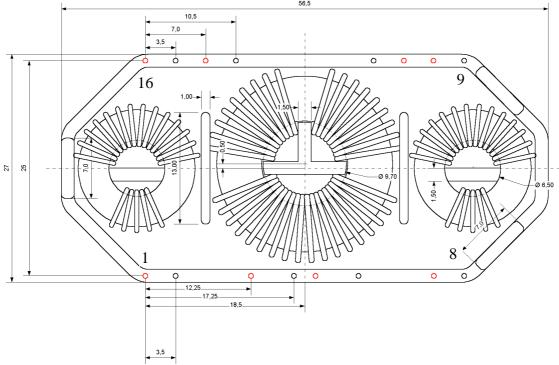
Figure 2.1 Complete transformers with cores in position
