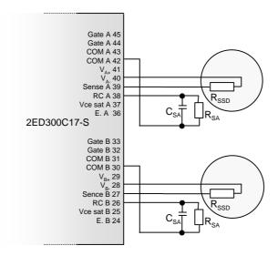
Figure 3.8.1 Connection of R<sub>SSD</sub>
